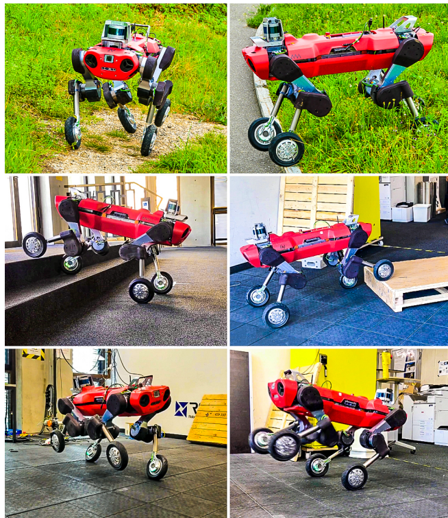
Fig. 1. With our novel whole-body MPC, the robot ANYmal [17], equipped with actuated wheels, explores indoor and outdoor environments in a fast and versatile way (video available at https://youtu.be/_rPvKlvyw2w ). First row: Locomotion in high grass and over steep hills of up to 2 m/s, while gait sequences are automatically discovered. Second row: Blindly stepping over a 0.20 m high step (32% of leg length) and stairs with a 0.175 m high step (28% of leg length). Third row: Pacing gait and 0.28 m high jump with front legs.
