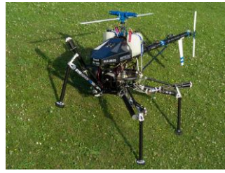
Fig. 11. Adaptive landing gear mounted on the Scout B1-100 to test the slip resistance
