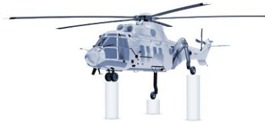
Fig. 16. Adaptive landing gear attached to the AS332 Super Puma in the preferable landing orientation
