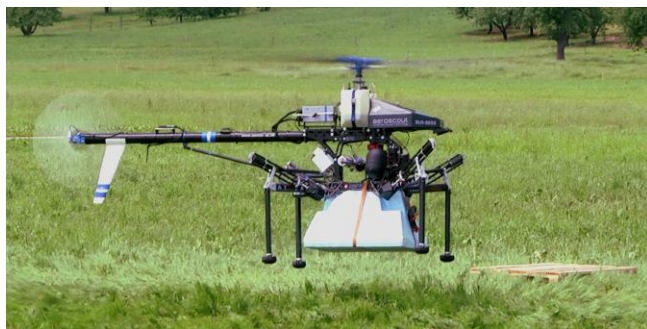
Fig. 12. Adaptive landing gear attached to the Scout B1-100 during a flight test next to the targeted obstacle
