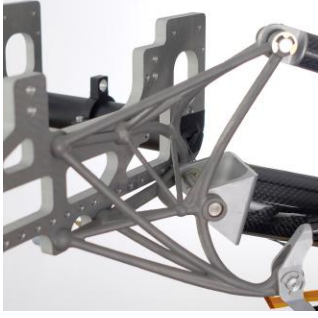
Fig. 7. Leg-fuselage interface including the helicopter chassis and leg
