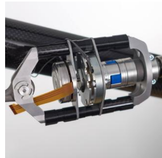
Fig. 5. Built-in actuation with cover removed showing the motor, brake and coupling (from left to right)
