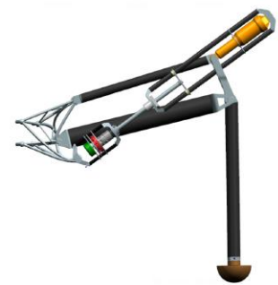
Fig. 3. Leg structure including the actuation, rods black, joints and spindle grey, brake red, damper yellow, motor green, foot brown
