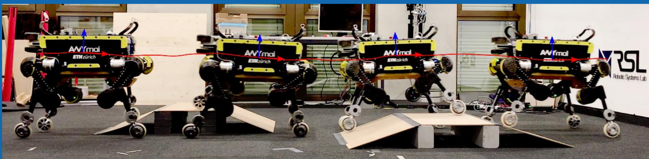
Fig. 1. The figure illustrates several skills of the wheeled version of ANYmal: dynamically driving down a step with 1 m/s (top left image), walking up a step (top right image), driving in a curve by yawing the base (lower left image), and dynamically driving down stairs with 1 m/s (lower right image).
